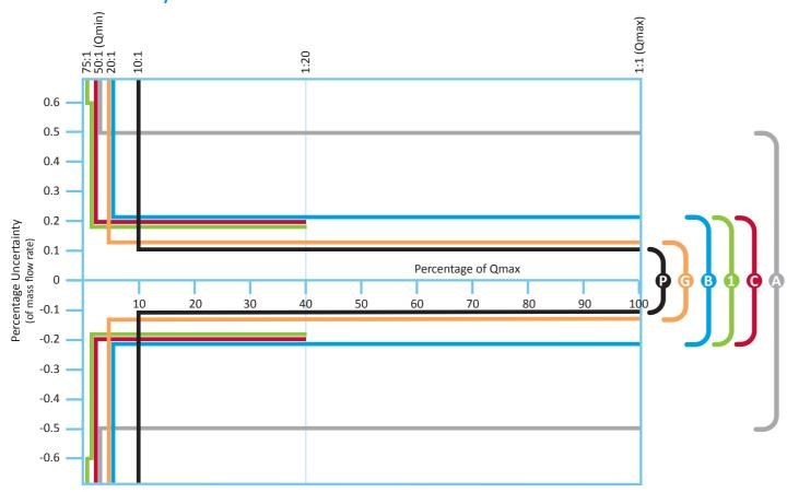
Only Rheonik offers a selection of calibration options to match application range for the best possible flow measurement performance. Select for wide turndown, higher accuracy or low flow optimized performance from the Rheonik calibration portfolio to maximize the value of your Rheonik Coriolis flow meter.
