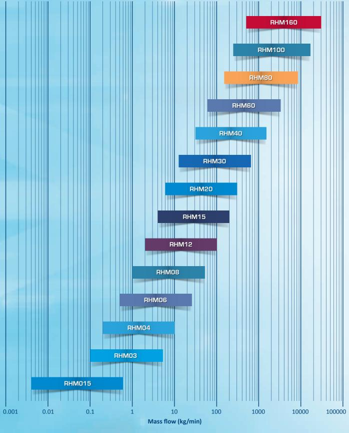
Flow rate chart depicts flow ranges for liquid applications at typical/common process pressure ratings. Flow ranges for meters with higher pressure ratings may vary. Gas flow ranges will depend upon pressure.
